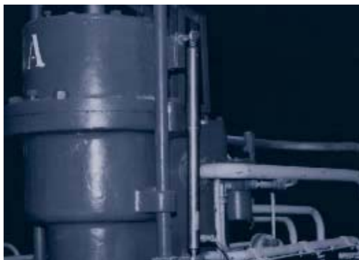
Heavy industrial LVDT monitoring valve position
