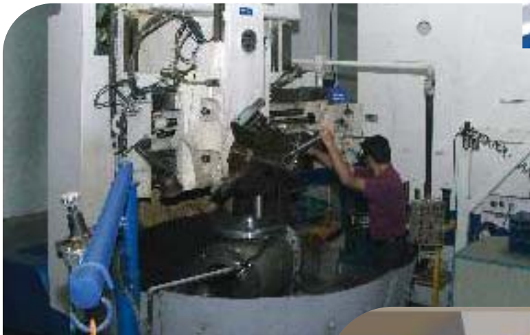
▲ Vertical Turning Lathe: for machining of bigger size valve bodies
