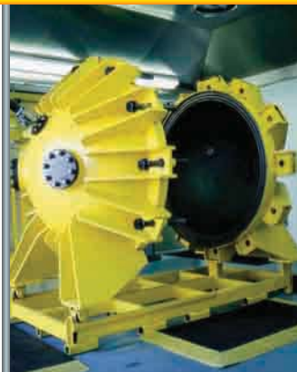
Standard ISO 1m 3 vessel for K_{ST} and P_{MAX} determination
